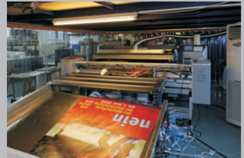
Interface between plotter and cutter. Optional dryer unit for solvent Ink.
